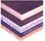
**SANDWICH** core panels consist of two thin advanced composite skins that 'sandwich' an ultra low density core such as foam or honeycomb. The surface finish of both skins is smooth and glossy as standard although a matte bonding surface can be specified if desired.
