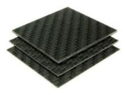
ECONOMY carbon fibre sheet is manufactured using multiple layers of genuine 100% 12k 2×2 carbon fibre twill reinforcements infused with epoxy resin creating a high stiffness, high strength, light weight and aesthetically pleasing material. All ECONOMY carbon fibre sheets have a glass transition temperature of 90°C with higher temperature performance available upon request. Other thicknesses and sizes available upon request.
