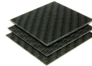
**ECONOMY** carbon fibre sheet is manufactured using multiple layers of genuine 100% 12k 2x2 carbon fibre twill reinforcements infused with epoxy resin creating a high stiffness, high strength, light weight and aesthetically pleasing material. All ECONOMY carbon fibre sheets have a glass transition temperature of 90°C with higher temperature performance available upon request. Other thicknesses and sizes available upon request.
