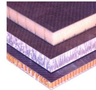
**SANDWICH** core panels consist of two thin advanced composite skins that 'sandwich' an ultra low density core such as foam or honeycomb. The surface finish of both skins is smooth and glossy as standard although a matte bonding surface can be specified if desired. Customised sandwich panel constructions are possible e.g. core type/density, skin materials, thickness and temperature performance.
